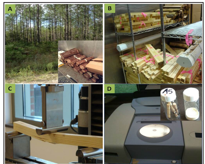
Figure 1. (A) Loblolly pine trees and bolts; (B) Test specimen for bending test; (C) Testing machine loaded with sample; (D) Test samples for NIR spectra collection
